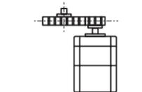
Connect the motor shaft to the center of gear teeth to be interlocked.
