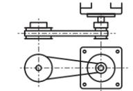
Connect the motor shaft and the line which connects the center of two pulleys to be perpendicular.
