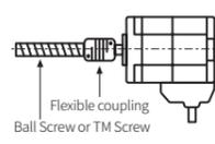
When connecting the load directly to the motor shaft, use a flexible coupling (ERB Series).
