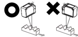
Install the emitter and receiver vertically to the line between crest and valley of the object.
