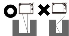
Install the sensor head where the reflected laser beam does not blocked toward the receiver part.
