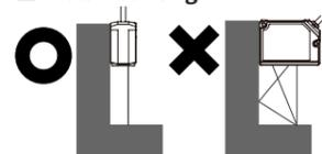
Install the sensor head where the reflected laser beam from the wall does not enter the receiver part. If the color of wall is black with low reflectivity and no gloss, the error can be minimized.
