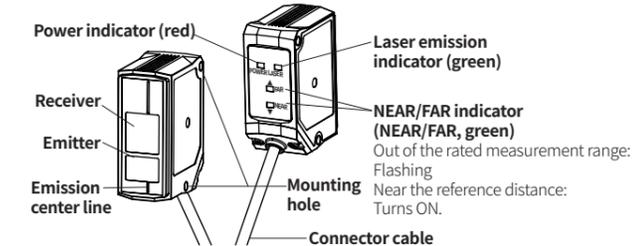
Emission center line and the object should be aligned because the laser is emitted along the line.
