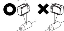
Install the emitter and receiver in parallel to the material or color boundary of the object.
