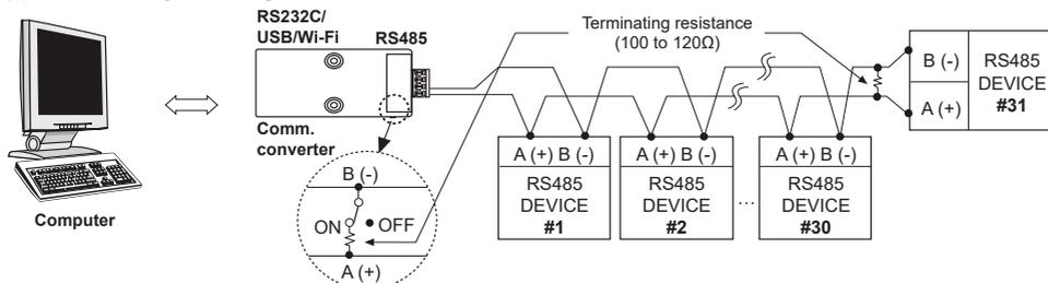
※It is recommended to use Autonics communication converter; SCM-WF48 (Wi-Fi to RS485·USB wireless communication converter, sold separately), SCM-US481 (USB to RS485 converter, sold separately), SCM-381 (RS232C to RS485 converter, sold separately). Please use twisted pair wire, which is suitable for RS485 communication, for SCM-WF48 and SCM-US481.
